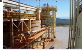
*Photo 6: Part of the lime neutralization high-density sludge acid mine drainage treatment plant at Minnesota Flats. The large tank at center-left is one of two in which acid mine drainage is mixed with lime slurry.*
